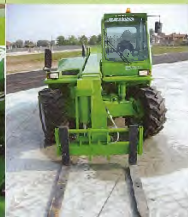
The 'disappearing' boom ensures an excellent 360° visibility.
