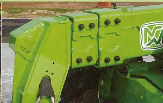
Boom sections slide on adjustable low-friction pads
